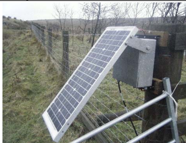
Solar panel: often used to power hydrometric networks, in this example an impress pressure transducer (water level recorder).
