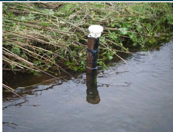
Water level recorder: measures temperature and pressure which converts into water level.
