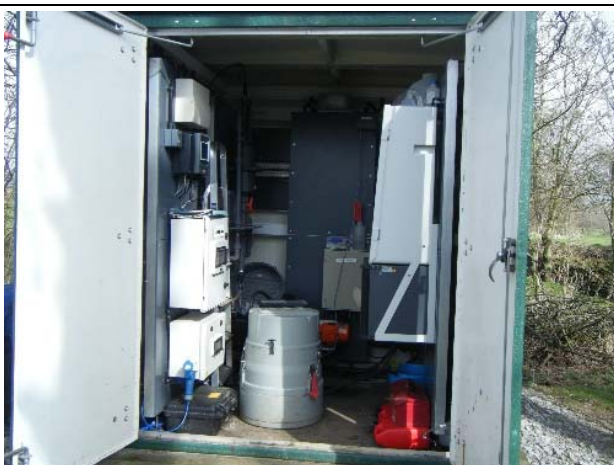
Water quality monitoring hut: built to house automatic water quality monitoring kit on site.
