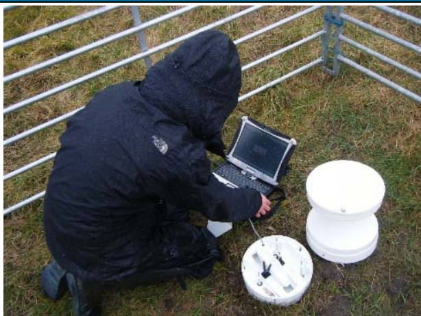
Rain gauge: a tipping bucket rain gauge is being programmed to measure rainfall every 2 minutes.
