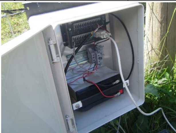
Logger box: telemetry system which uses a 'machine to machine' (M2M) data SIM card to transmit and receive data via the internet.
