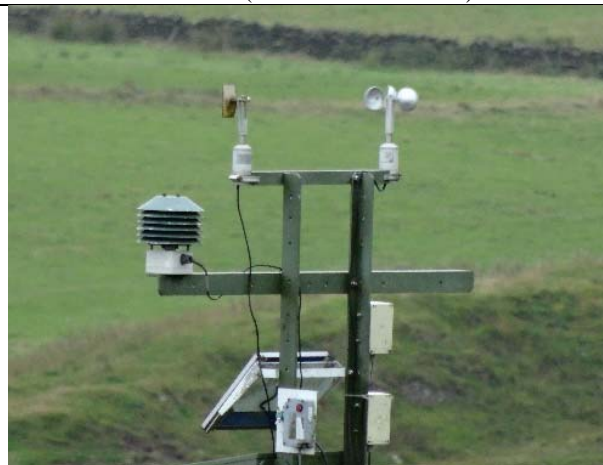
Weather station: an automatic weather station monitoring many parameters e.g. wind speed
