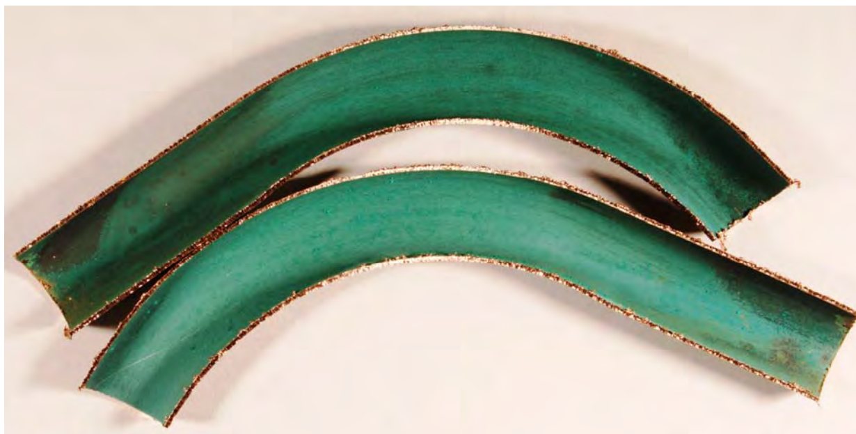
Figure 1 Stable continuous malachite layer on bore of copper cold water pipe © P Munn
