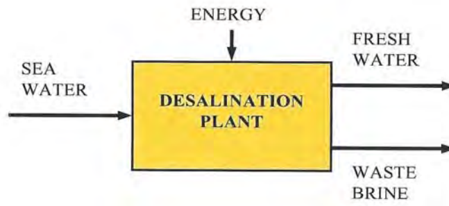
Figure 5: Basic principle of desalination.
