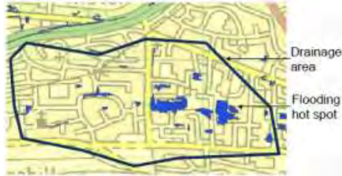
Proactive investigation of sewer flooding hot spots
